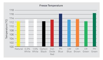
Figure 4. Freeze temperature test results
