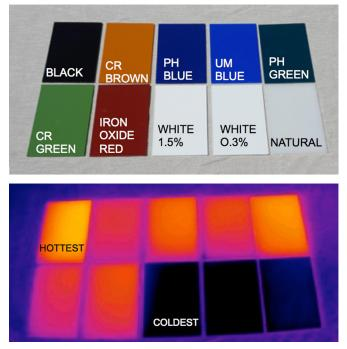
Figure 7. Thermal imaging of different pigments
