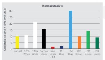
Figure 6. Thermal stability/surface oxidation test results
