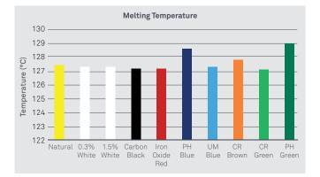
Figure 3. Melt temperature test results
